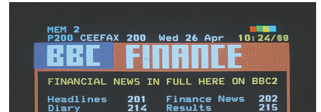
A Teletext page with the colour bar at the top right indicating that it is a Fastext page.
